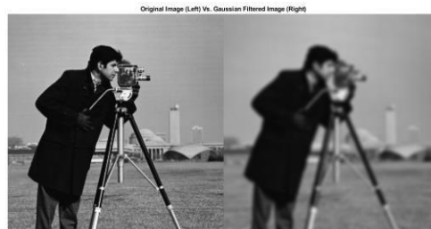
Figure 3. Gaussian Filter applied on an image
