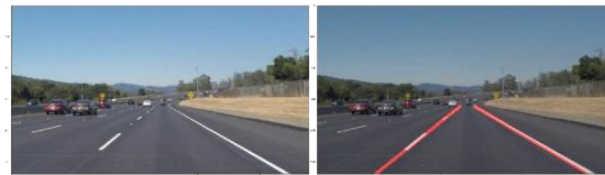
Figure 6. Final image after detection of lane and line
