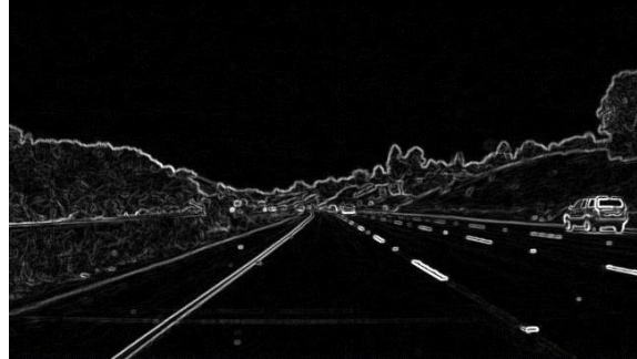
Figure 4. Image obtained after Canny edge detection.
